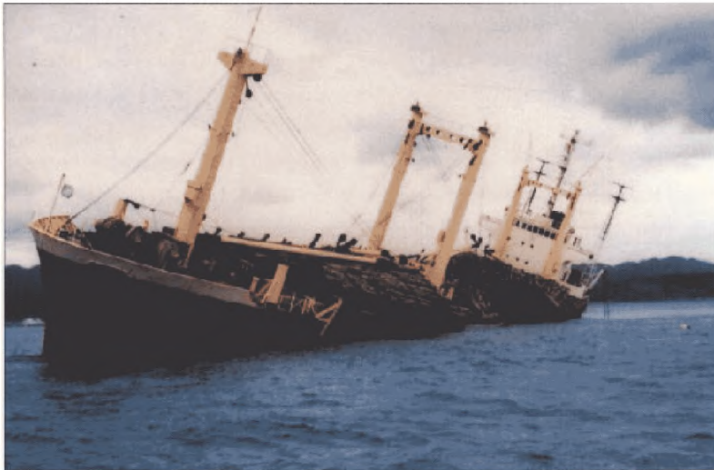
Photograph 2 Timber carrier listing due to ingress of water
